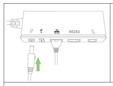
3. Plug the barrel connector of the power cable into the port on the multi-port box labelled with the power symbol (  $\checkmark$  ).
