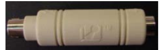
Figure 4: Keycatcher - this is a device that can be connected to a keyboard to record all the keystrokes.
