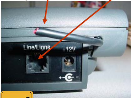
Figure 5A: Unauthorized external cable/broken port.
