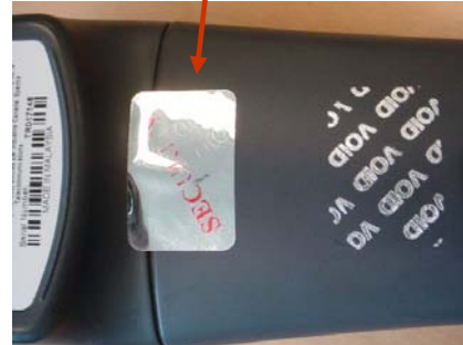
Figure 5C: After removal of security seal.
