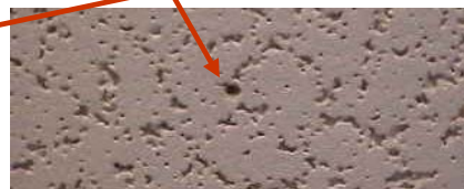
Figure 5B: Tampered security seal.
