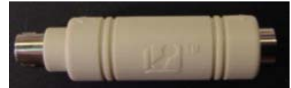
Figure 4: Keycatcher - this is a device that can be connected to a keyboard to record all the keystrokes.
