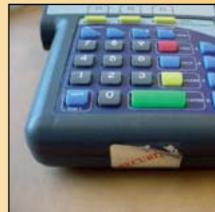
Tampered security seal
