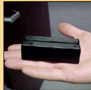
Card skimming devices used to copy the magnetic stripe information are tiny and can even be carried by employees.
