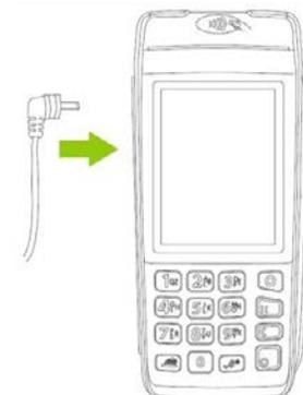
3. Insert the direct-to-terminal cable connector into the port.
