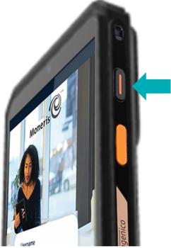
A photograph of the Moneris Go Slim Integrated terminal. A teal arrow points to the power button on the right side of the device. | <ol style="list-style-type: none"><li>1. Press and hold the &lt;Power&gt; button on the right side of the terminal for more than 2 seconds until the menu panel appears.</li></ol> |
