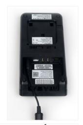
4. Make sure the AC adaptor is connected to the other end of the charging cable. Plug the AC adaptor into a working electrical outlet.
