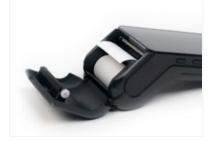
4. Close the printer cover and press down to snap it back into place so that the extended paper is held securely.
