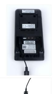
2. Turn the communication base upside down. Use one end of the cable and insert it into the Ethernet port on the back of the base. The Ethernet cable will clip in when it is inserted correctly.
