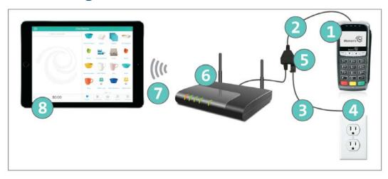
**Note:** You must use the exact power adaptor and cables provided by Moneris to work with the iPP320 PIN Pad. Failure to do so may affect the operability of, or cause damage to, the equipment.
