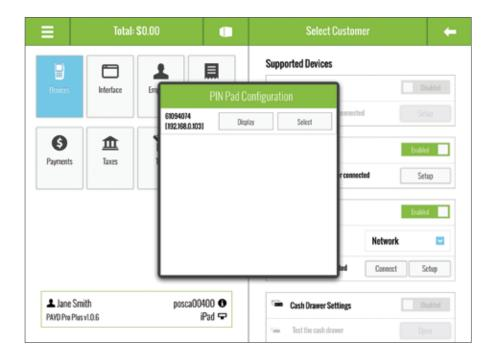
10. Match the ID shown in the PIN Pad Configuration popup with the ID on the iPP320 PIN Pad's display screen.
