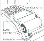
d. Close the lid, and press down to snap it back into place so that the extended paper is pressed securely against the closed lid and the faceplate.
