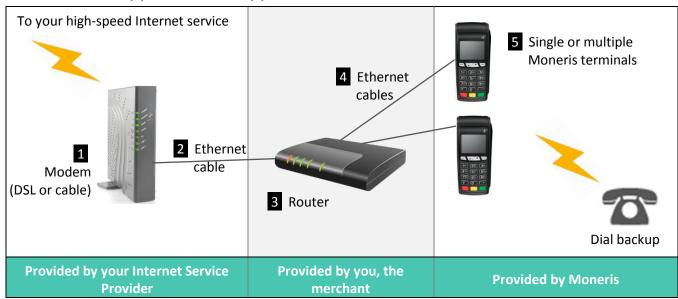
**Note:** The Moneris iCT250 is used in this diagram as an example. This diagram is applicable to all of the terminals listed on page 1.
