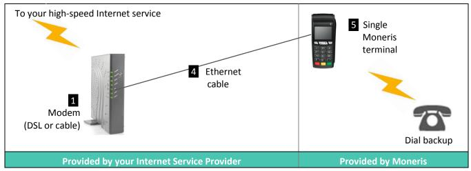
**Note:** The Moneris iCT250 is used in this diagram as an example. This diagram is applicable to all of the terminals listed on page 1.
