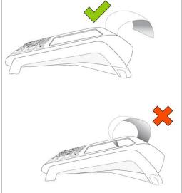
4. Close the lid, and press down to snap it back into place so that the extended paper is pressed securely against the closed lid and the faceplate.
