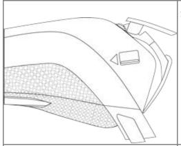
1. Lift the printer latch up, and then pull back to open the lid and expose the paper well.
