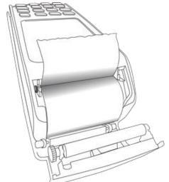
2. Insert the paper roll into the paper well with the loose end unrolling from the bottom of the roll toward the back of the terminal.
