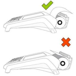
2. Insert the paper roll into the paper well with the loose end unrolling from the top of the roll toward the back of the terminal.
