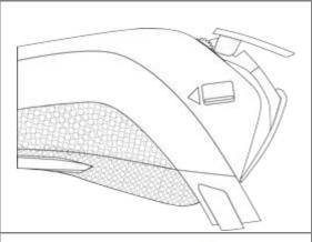
1. Lift the printer latch up, and then pull back to open the lid and expose the paper well.
